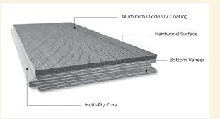
The manufacturing of Engineered Flooring is typically more resource efficient and cost effective.
